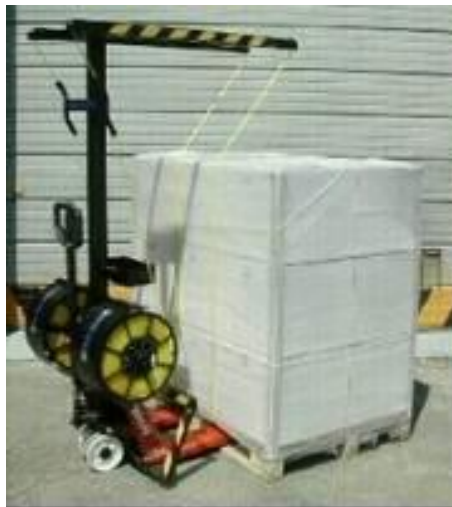
Figure 7 – Application of the Pallet Strapping
