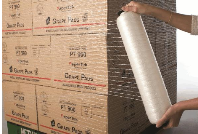
Figure 6 – Wrapping Film (Stretch Film) Technique
