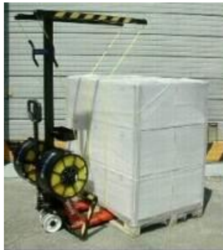
Figure 7 – Application of the Pallet Strapping
